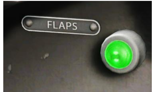
Flaps Mechanical Indicator (Shown Deployed)
