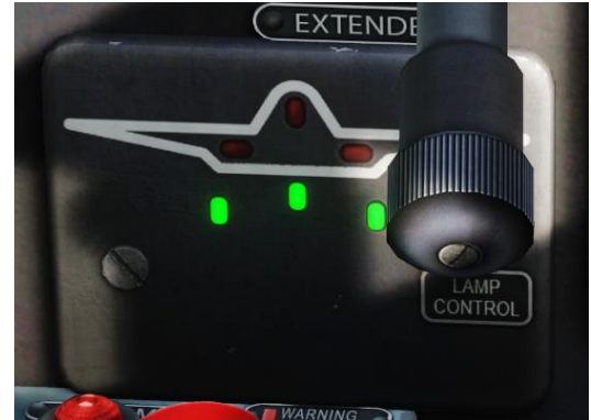
Main Landing Gear Mechanical Indicator (Shown Deployed)
