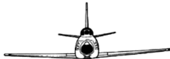
Wingspan of a F-86 Sabre: 11 m (Value to enter in gunsight wingspan)
