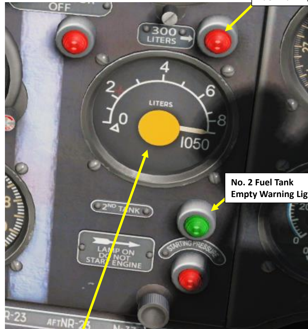
300 L Remaining Fuel Warning Light
